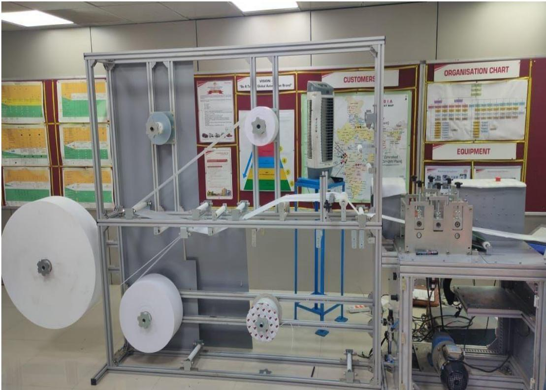
**Swachh 7.0** is a fully-automatic machine for producing 3 ply surgical masks.
